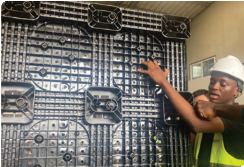
New pallet produced by Namé from recycled plastic
